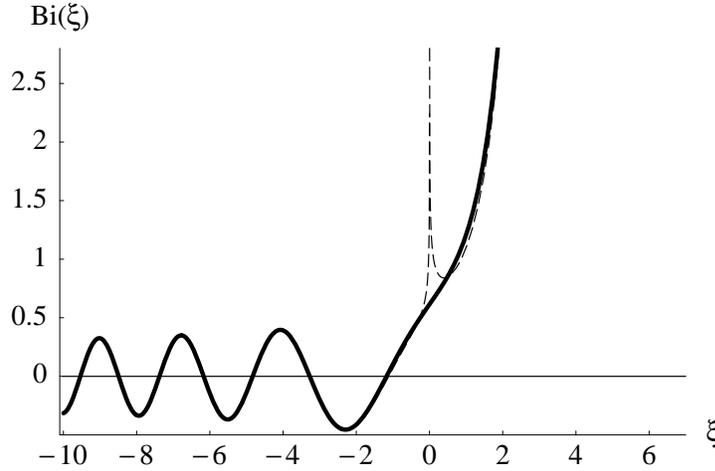
Figure 1.8: The AIRY function  $\text{Bi}(x)$  (solid curve) and its asymptotic forms (dashed curves).
